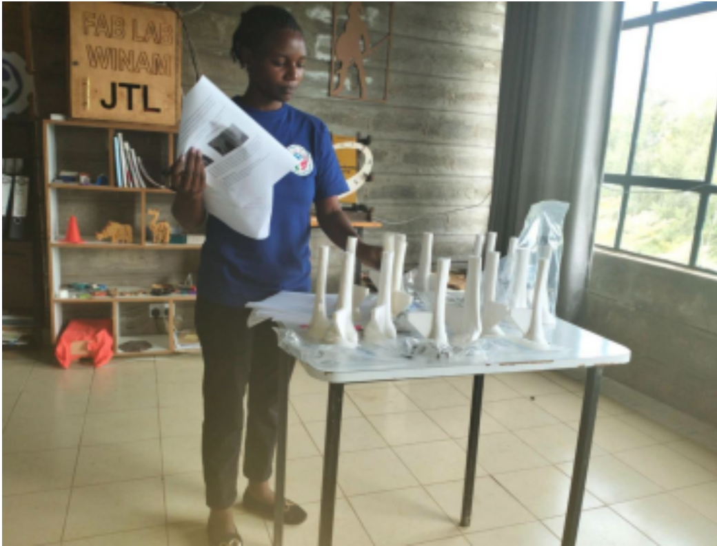
Picture 4. Quality inspection of tibial fracture fixators produced at FabLab Winam, Kisumu, Kenya (Nov. 2023)
